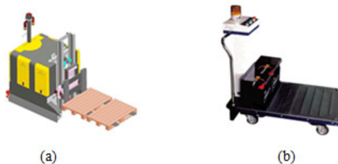
Figura 3.2. Tipos de AGVs: (a) carga de pallet (ELETTRIC80, 2009), (b) cargas leves (AUTOMOTION, 2009)
