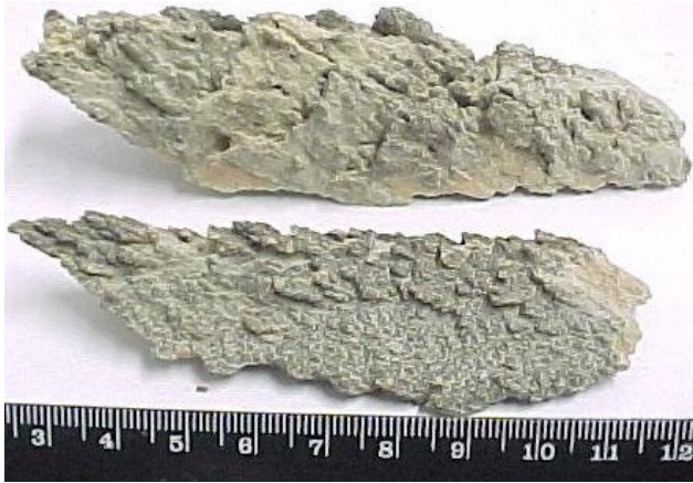
Figure 3.1 – A typical ash deposit from the superheater of Jorge Lacerda thermo power plant. The scale is marked in mm.
