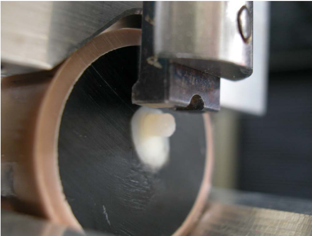
Figure 1 – Cylinder-shaped acrylic resin base attached perpendicularly to dentin surface. Close-up view of the blade in position for the shear-bond.
