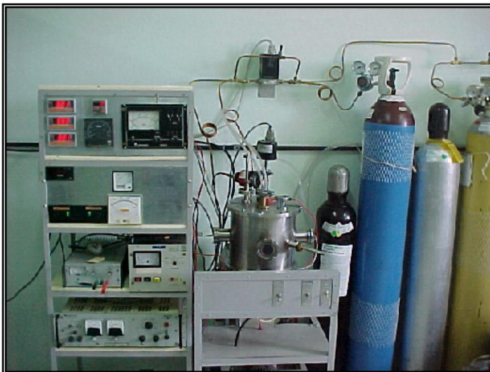
Figura 16: Reator a plasma de Magnetron Sputtering.
