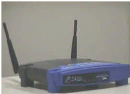
FIGURA 8: Wireless Network Access Point
