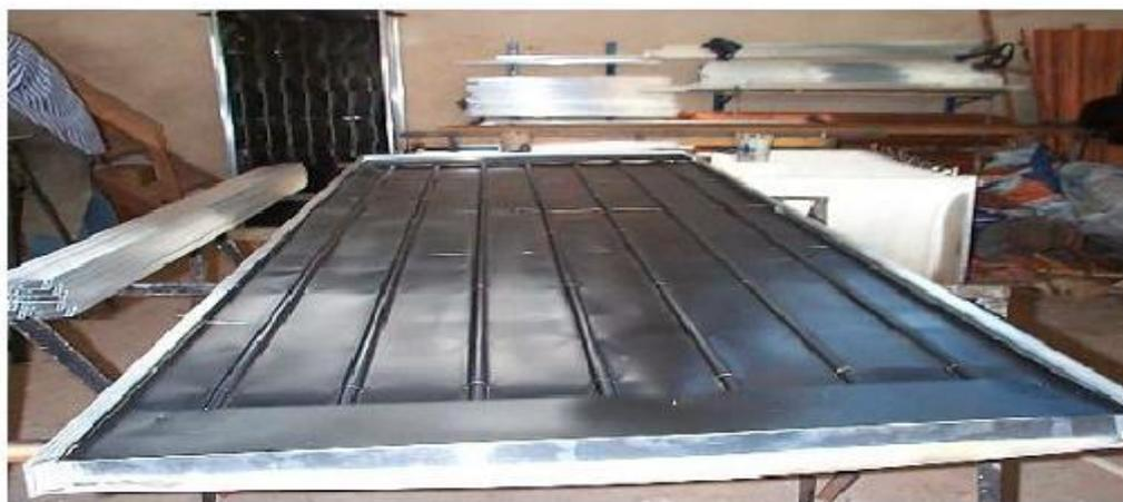
**FIG. 3.2 FOTO DA MONTAGEM DA PLACA COLETORA VERTICAL .**
