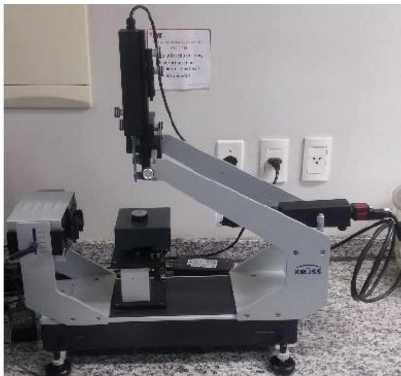
Figure 11 – Goniometer used for contact angle measurements.
