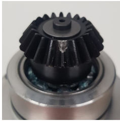
(a) Pinion with a chipped tooth
