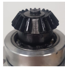
(b) Pinion with a missing tooth
