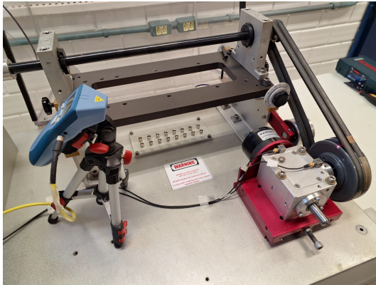
(a) Tachometer pointed at the pinion pulley
