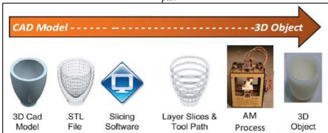
Figure 10 - Main steps in additive manufacturing: From CAD modeling to final 3D printed part
