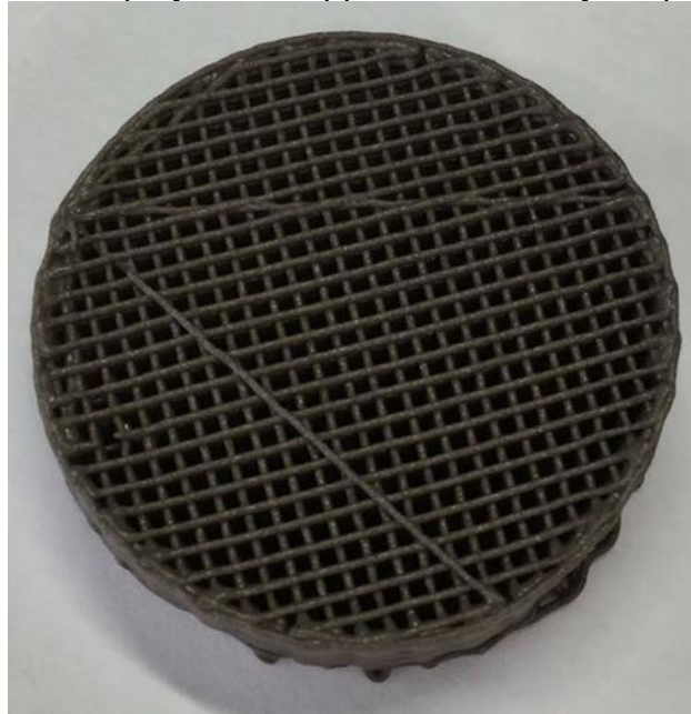
Figure 8 Geopolymeric support obtained by 3D printing.
