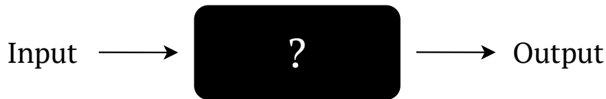
Figure 5 – Black box function: a function where only the input and output values are known, but not its expression.
