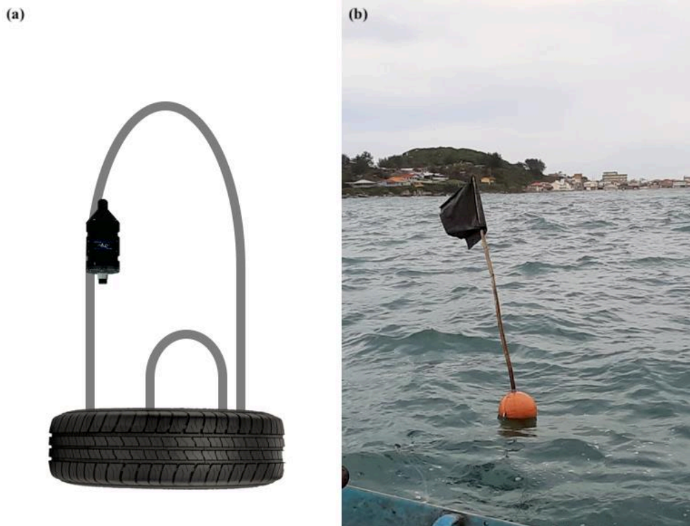
Figure 4 – (a) Layout of the mooring used, with the SoundTrap attached to the taller loop; (b) Buoy used to mark the recorder's position.
