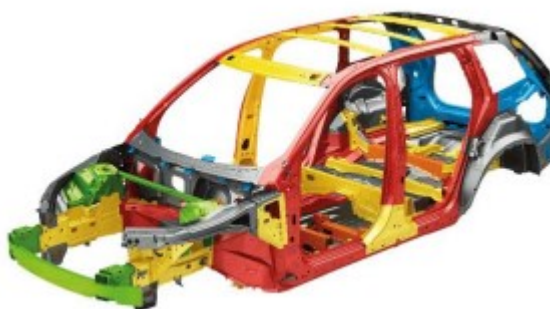
Figura 21 – Chassis Unibody do Volvo XC90
