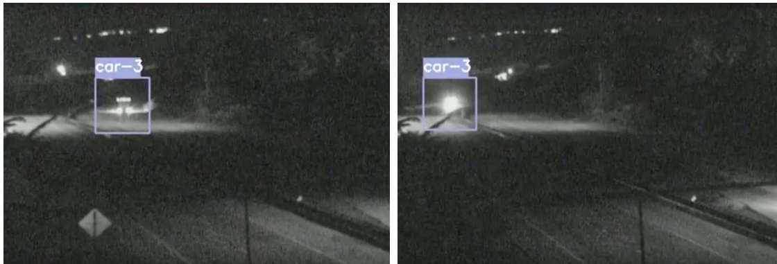
Figure 4.4: Tracking error sample: Same ID for two different vehicles. Source: Author
