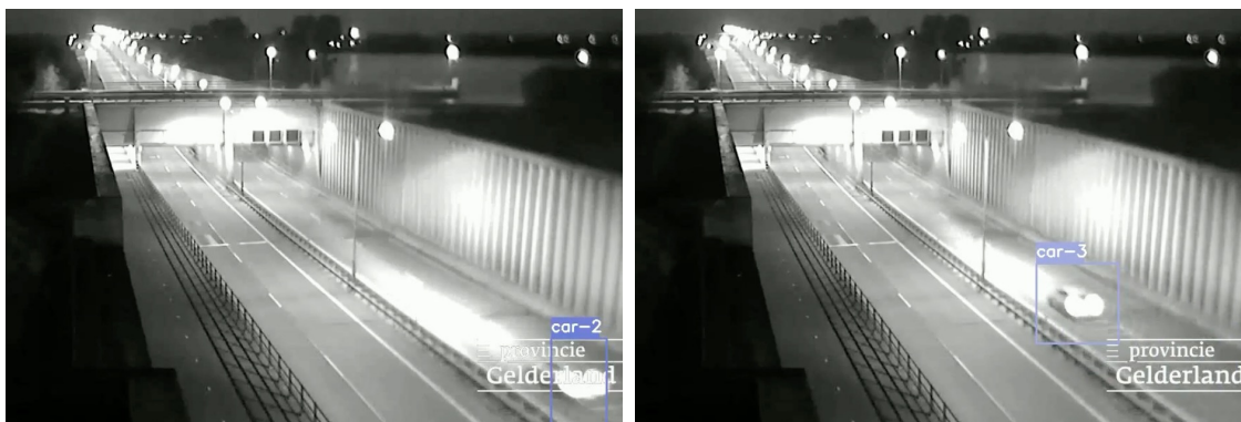
Figure 4.5: Tracking error sample: Occlusion by objects Source: Author
