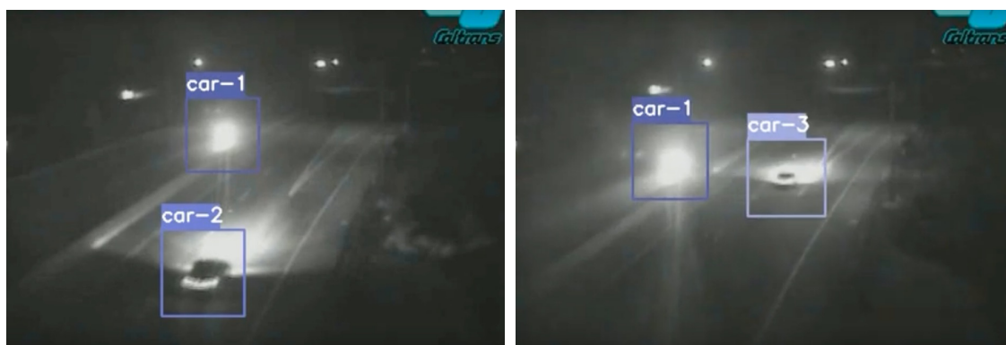
Figure 4.3: Tracking error sample: Lost of bounding box. Source: Author
