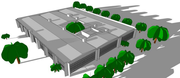
Figure 31 – Building 02’s rooftop and N surface shadings at 6:00 a.m. in December.
