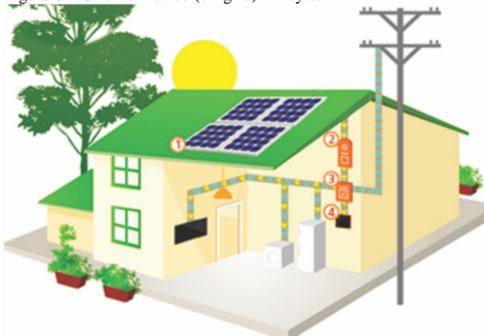
Figure 6 – Grid-connected (on-grid) PV system.
