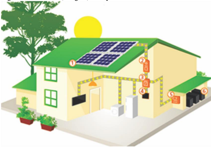
Figure 5 – Isolated (off-grid) PV system.
