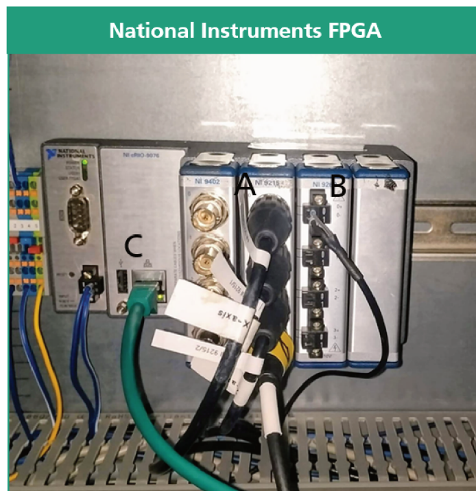
Figure 30 – FPGA A- Acquisition Module; B- Control Module; C- Ethernet Communication
