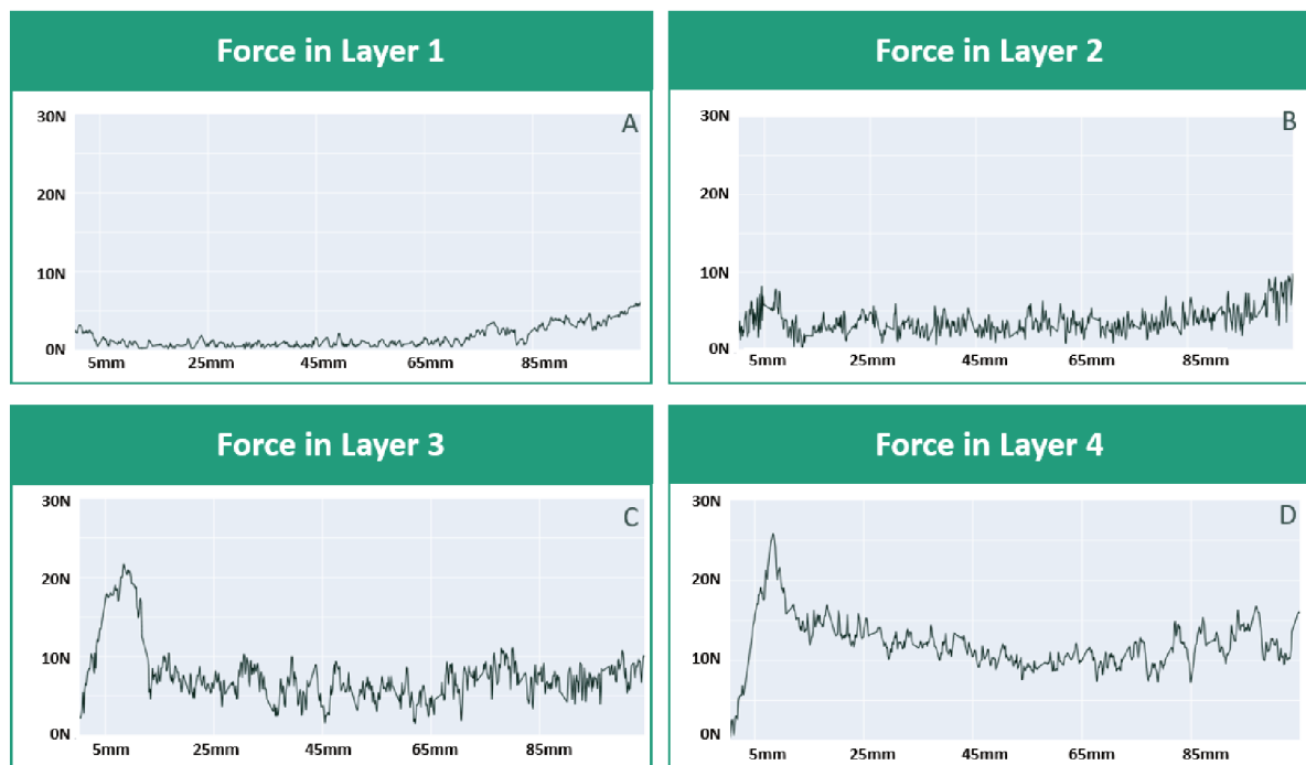
Figure 12 – Comparison between the dynamics through multiple layers
