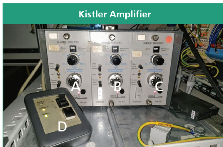
Figure 29 – Hardware used for transforming force into voltages
