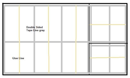
Figure 8 – Schematics on double sided tape and glue line to glue reflexive the sheet on the cardboard. Source: The authors
