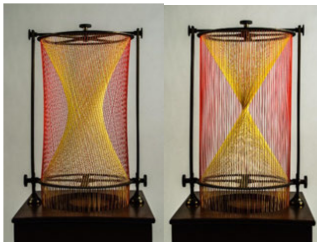
Fig. 6, 7. The model shown in fig. 3 has a movable upper ring. Turning the upper ring leads to the depiction of two different hyperboloids: the inner hyperboloid (lighter strings) becomes more and more closed, until a cone, and the outer hyperboloid becomes more open, until a cylinder (Museum of ISEP MPL321OBJ)
