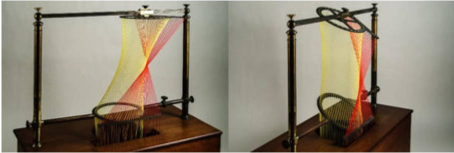
Fig. 12, 13. Idem. We can also move the lower brass bar, so that the cone, cylinder and hyperboloids may be straight or oblique (Museum of ISEP, MPL308OBJ)
