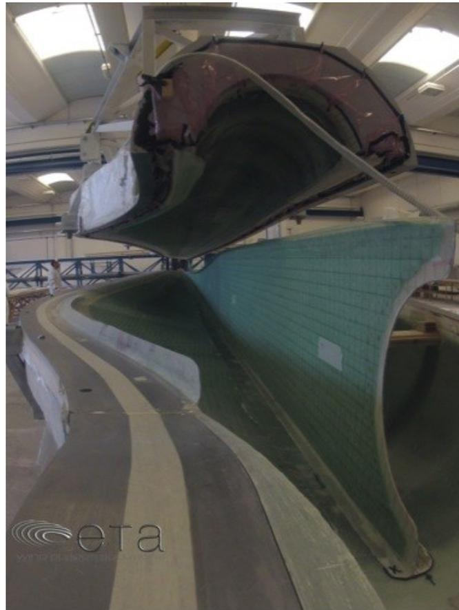
The two shells of a 60kW blade being joined
