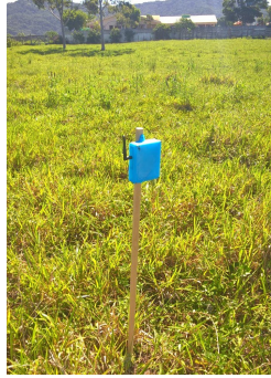
Figure 7.9: Positioning anchor deployed on the test field Source: Original
