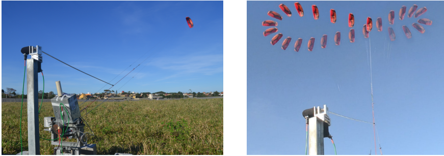
Figure 7.11: Small scale prototype and time lapse of the kite trajectory Source: Original
