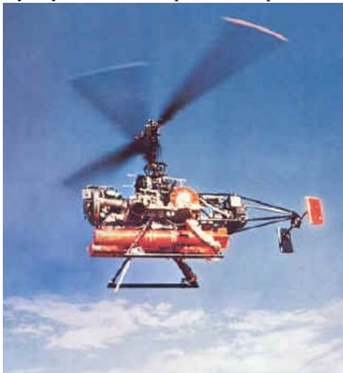
Figura 2 – Gyrodyne DASH transportando torpedos anti-submarino.
