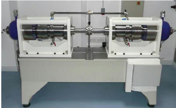
Figure 4.4: Rapid compression machine at C3 - National University of Ireland, Galway.
