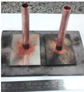
Figure 64 - Evaporator LHP preparation for sintered process of copper powder.
