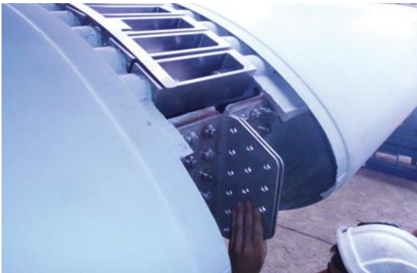
Figure 2.8 – Metallic fittings are bonded into the spar laminate of each blade segment and then bolted together to join the two segments. (Source: Gamesa [26])
