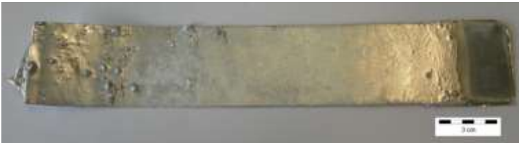
Figure 42 – Cold rolled sample after immersion in aluminium melt at 900°C for 15 s
