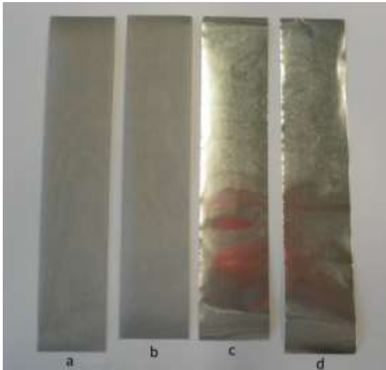
Figure 25 – Nickel mesh a) 150 mm-long b) 145 mm-long and aluminium foil c) 145 mm-long and d) 150 mm-long stripes
