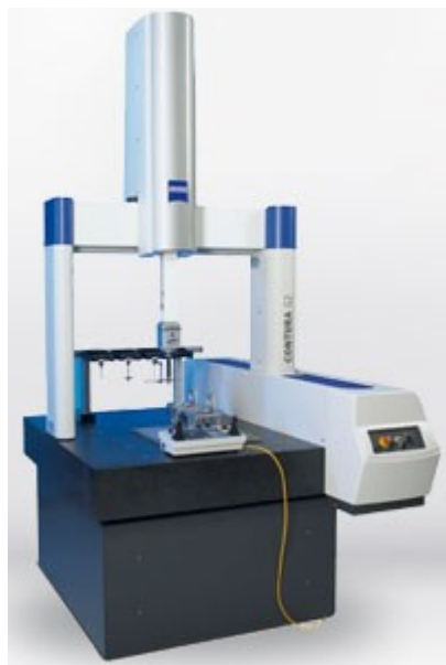
Figure 1.1: Tactile CMM measurement system [1].
