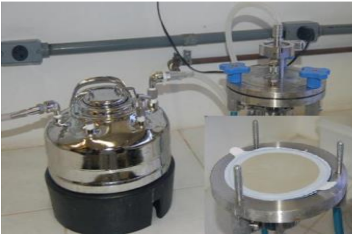
Figure 14: Vacuum filtration system with a capacity of 5L water, used for viral concentration.
