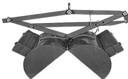
Figure 13: Petersen grab dredge used for sediment sample collection
