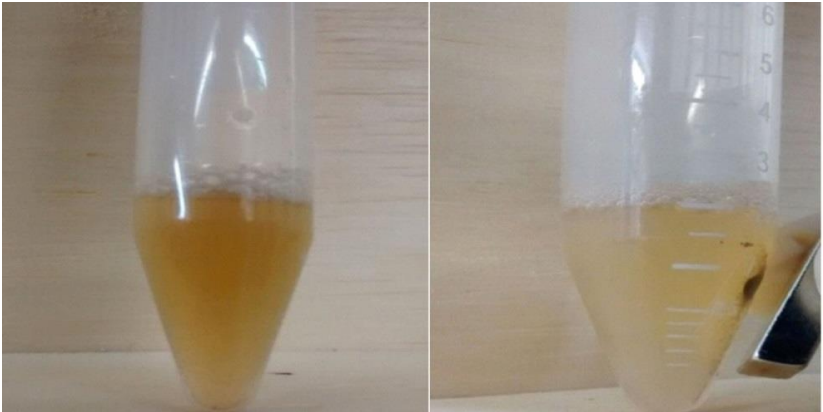
Figure 7 MNPs-PMMA nanoparticles in PBS (7.4) without application of an external magnetic field and with application of an external magnetic field.
