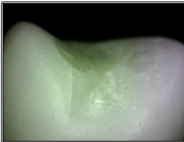
Fig. 7 – Survived specimen demonstrating the degradation (cracks) of the CAD/CAM crown similar to that observed in vivo .
