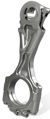
Figure 20: Concept of FEV two-stage VCR connecting rod. The compression ratio actuation is made only by the connecting rod, which contains the eccentric link and the hydraulic pistons to change the position of the piston pin. (FEV, 2015)
