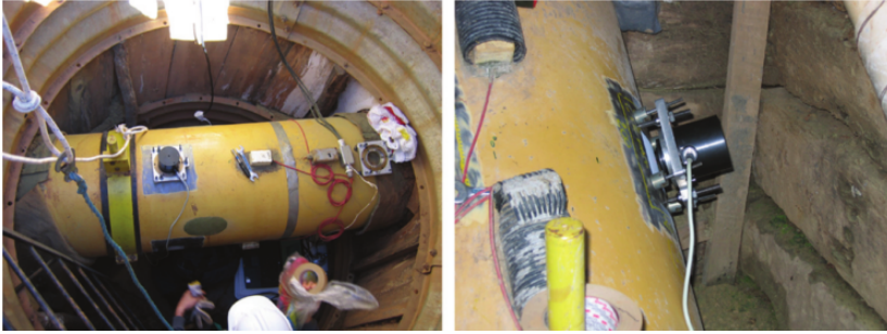
Figure 1.1 – In-field measurement of combined stresses in two gas pipeline cross-sections [6].
