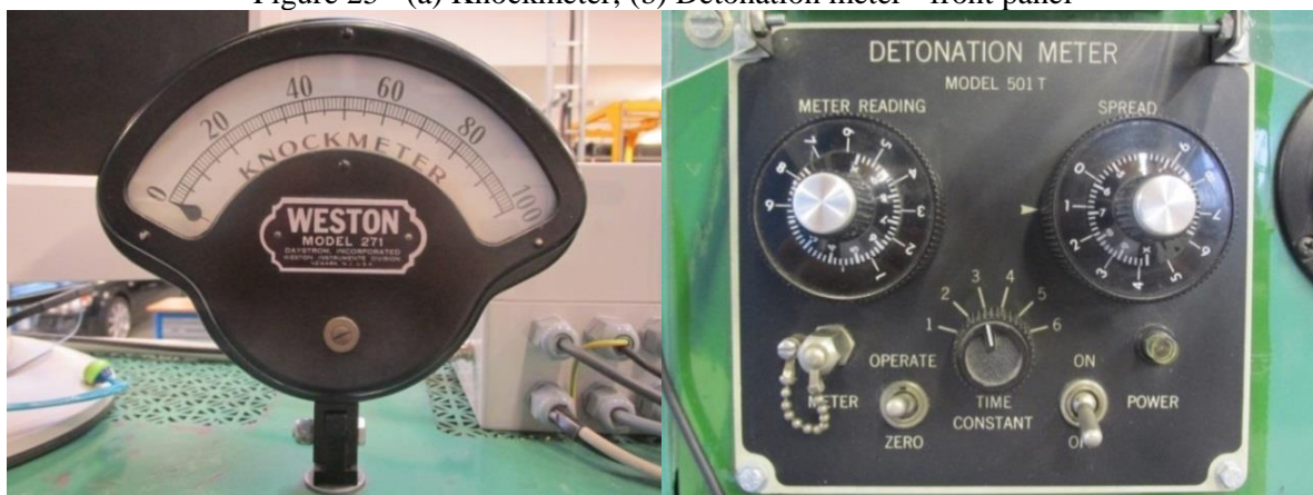
Figure 25 - (a) Knockmeter; (b) Detonation meter - front panel
