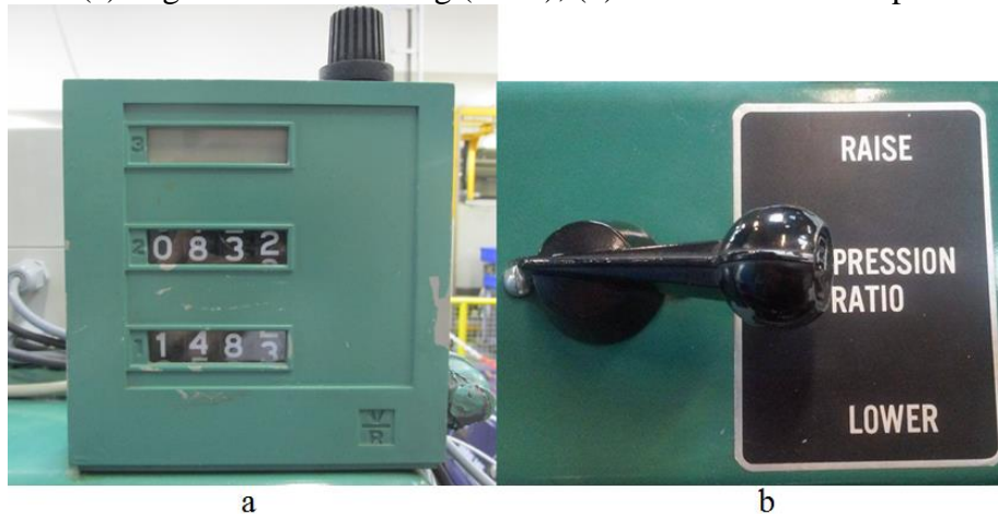
Figure 26 - (a) Digital counter reading (DCR); (b) Hand crank to compression ratio.
