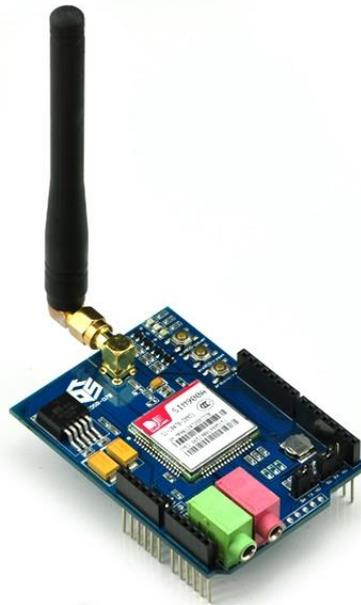
Figura 9 – *Shield* GSM (TINYSINE, 2016).
