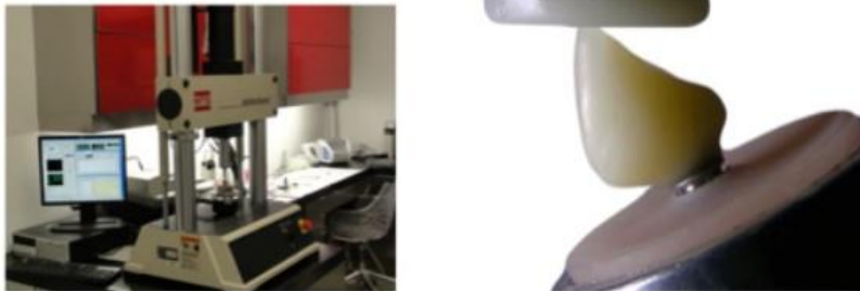
Figure 4. (A) Closed-loop servo hydraulic system (Mini Bionix II). (B) View of the specimen under load application.
