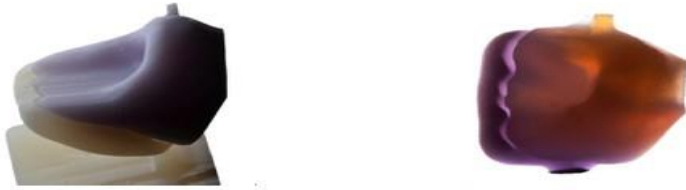
Figure 2. (A) Dentin-shaped lithium disilicate (Emax) mesostructure with a nano-filled composite resin veneer (Lava Ultimate) (group CEL). (B) Dentin-shaped nanofilled composite resin (Lava Ultimate) mesostructure with a lithium disilicate veneer (Emax) (group CLE)
