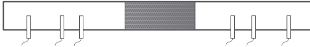
Figure C.1 – Schematic representation of the test duct with microphones before and after the liner sample.
