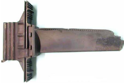
Figure 2.17 – Damaged turbine blade.
