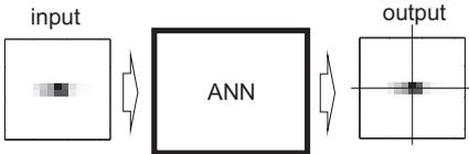
**Figure 5.** The inputs of the ANN are the subaperture image pixels. The outputs are the x and y position of the real centre. To train the ANN the outputs are provided with the inputs; when being used, the ANN should generate the correct outputs automatically.
