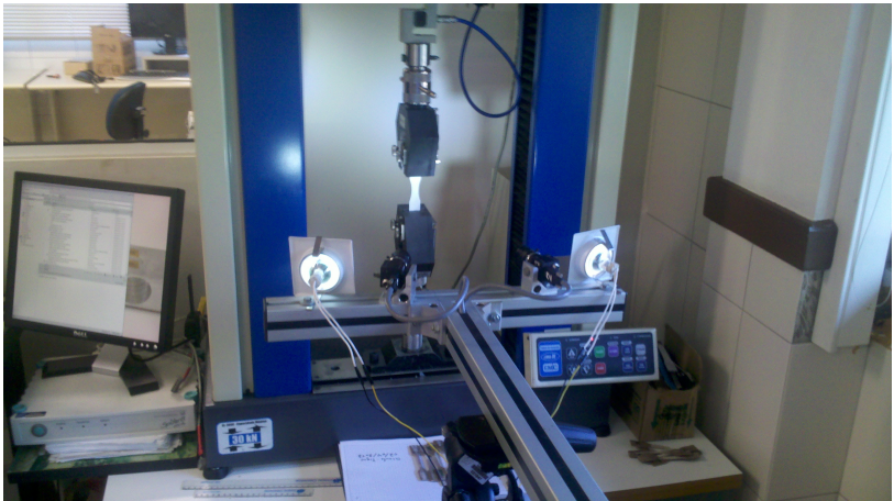
Figure A.1: The DIC apparatus and the test machine.
