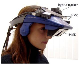
Figura 2.15: See-through head mounted display (HMD).
