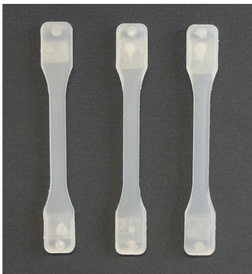
Figure 6.2: Samples of the specimens used in the tensile and Poisson's ratio tests.
