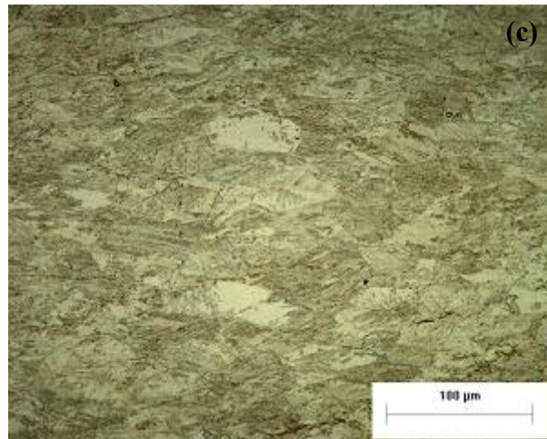
Figura 4.7: Micrografias do AIA 304 H (a) com \epsilon_{eq}=0.052 , (b), \epsilon_{eq}=0.21 , (c) \epsilon_{eq}=0.44
