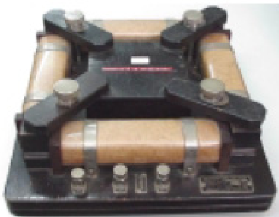
Figura 3.2 - O quadro de Epstein (B-EP-25cm da Yokogawa Electric Works Ltda)
