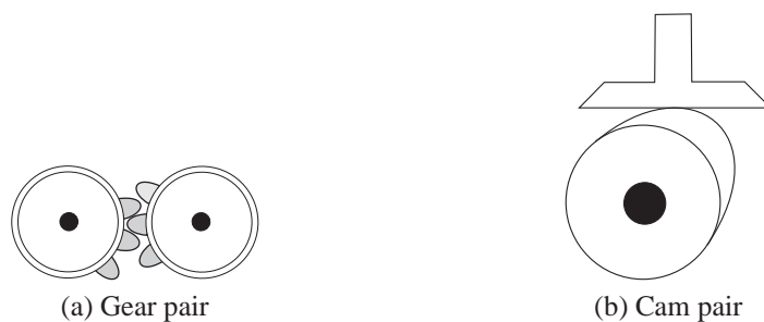
Figure 2.2: Frequently used higher kinematic pairs
