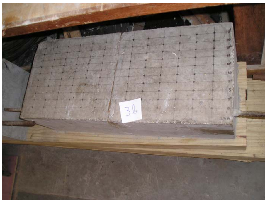
Figura 4.14 – Molde 3b (h=10,0 cm; \omega =6 mm; \phi =12,5 mm).
