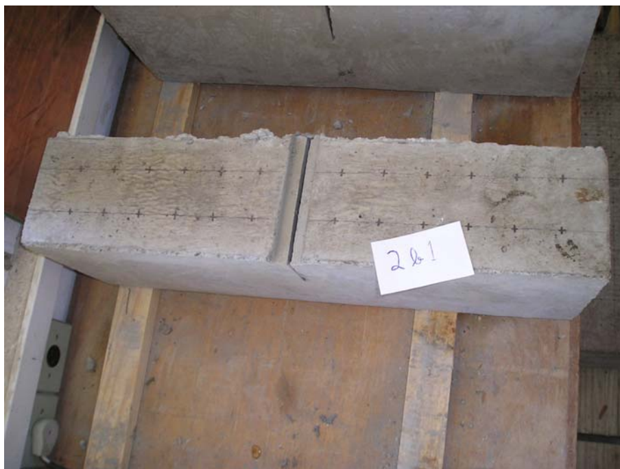
Figura 4.12 – Molde 2b1 ( h=10,0 cm; \omega=6 mm).
