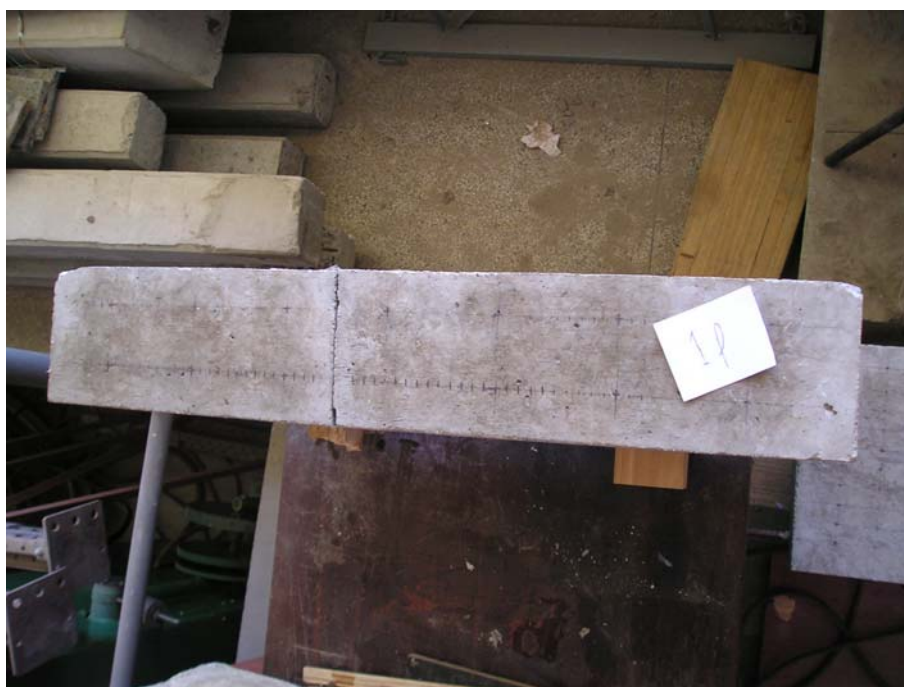
Figura 4.9 – Molde 1f ( h=22,0 cm; \omega=3 mm).
