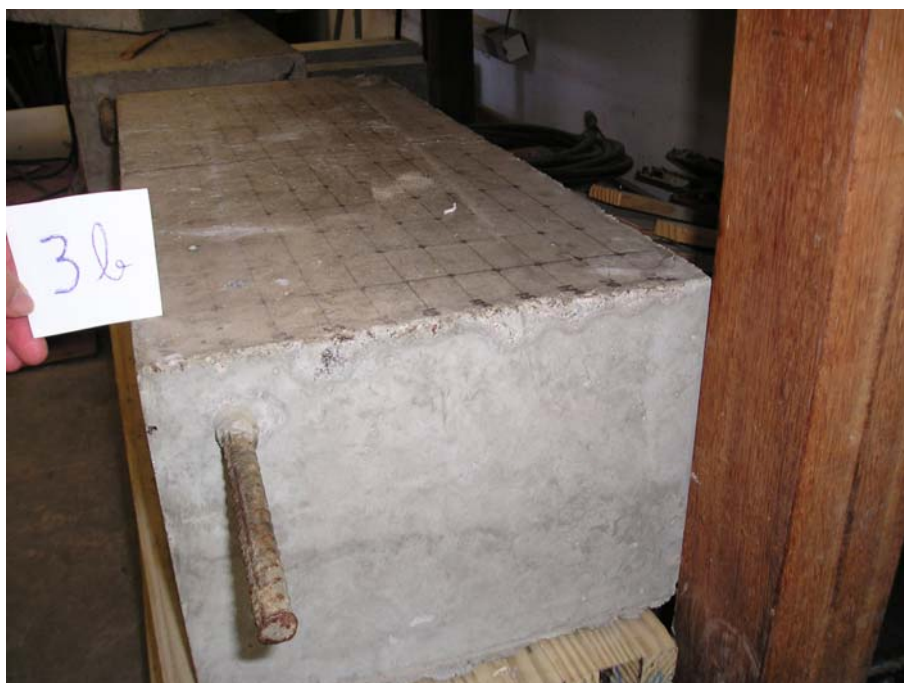
Figura 4.15 – Molde 3b (h=10,0 cm; \omega =6 mm; \phi =12,5 mm).
