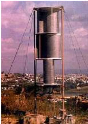
Figura 3.13. Rotor Savonius
