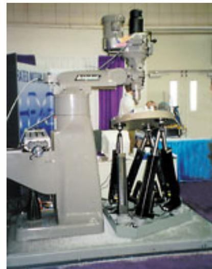
Figura 2.8 – Máquinas-ferramenta Hexapod [35, 36].
