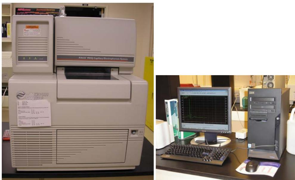
**Figura 2.** Equipamento Beckman Coulter P/ACE MDQ (San Ramon, CA) acoplado a software 32 Karat<sup>®</sup> (Beckman Coulter)
