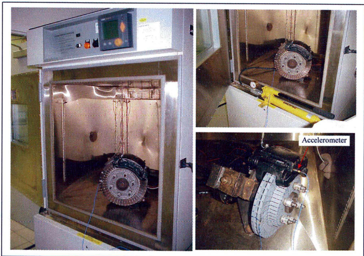
Figure 6.1 – Pictures of the setup for measurements of the brake system under temperature
