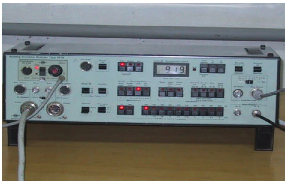
Figura 10 : Analisador ( Building Acoustics Analyzer 4418 da B&K).
