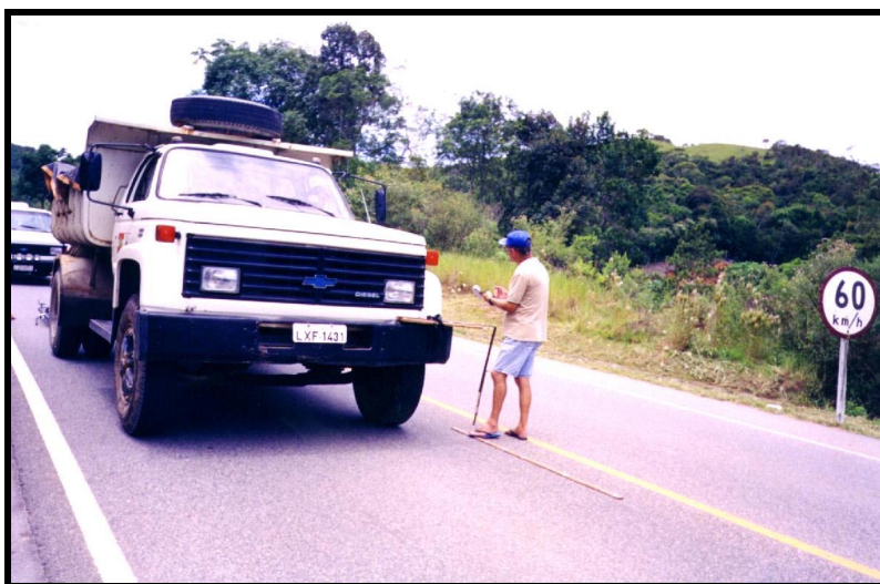
FIGURA 3.11 -Levantamento com a viga Benkelman - DNER-PRO-024/94
